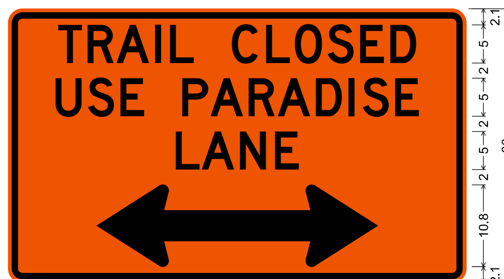
1.9" Radius, 0.8" Border, 0.5" Indent, Black on, Orange; "TRAIL CLOSED", D 2K; "USE PARADISE", D 2K; "LANE", D 2K; Standard Arrow Custom 28.0" X 10.8" 180' Black;
