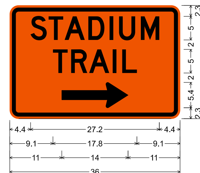
1.9" Radius, 0.8" Border, 0.5" Indent, Black on, Orange; "STADIUM", D 2K; "TRAIL", D 2K; Standard Arrow Custom 14.0" X 5.4" 180' Black;
