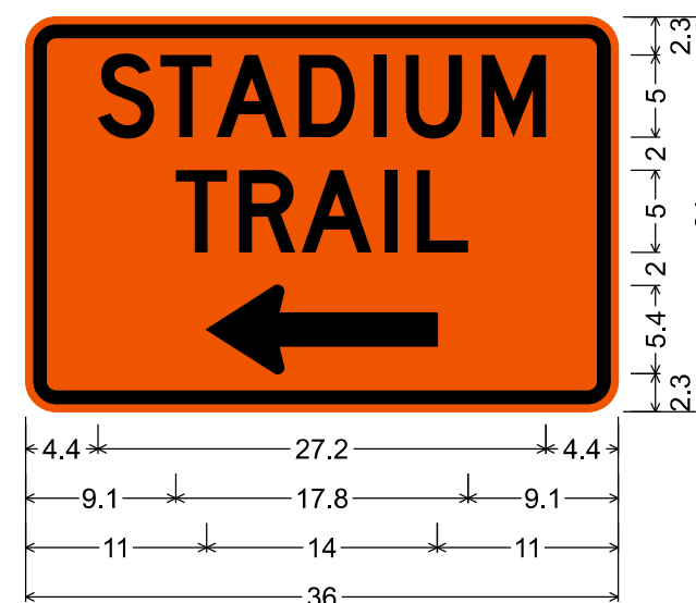
1.9" Radius, 0.8" Border, 0.5" Indent, Black on, Orange; "STADIUM", D 2K; "TRAIL", D 2K; Standard Arrow Custom 14.0" X 5.4" 180';
