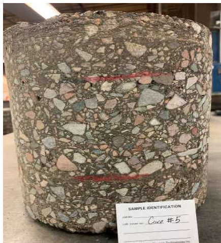
B5 Core Thickness: 9.0-in Top: 2.1-in, Middle 3.8-in, Bottom: 3.1-in.
