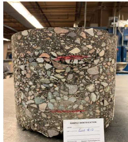
B12 Core Thickness: 8.3-in Top: 2.1-in, Middle 3.9-in, Bottom: 2.3-in.
