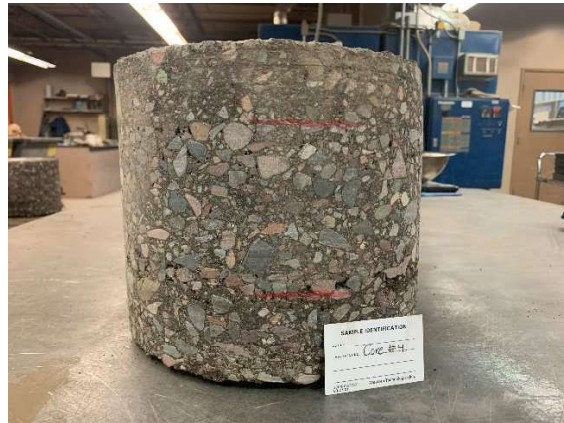
B4 Core Thickness: 8.5-in Top: 1.8-in, Middle 4.2-in, Bottom: 2.5-in.
