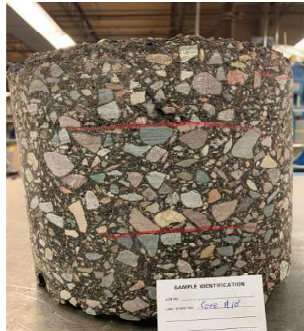
B18 Core Thickness: 8.5-in Top: 2.3-in, Middle 3.1-in, Bottom: 3.1-in.
