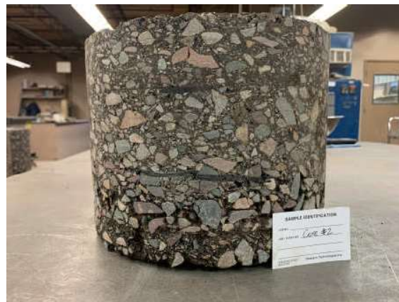
B2 Core Thickness: 7.9-in Top: 1.9-in, Middle 2.9-in, Bottom: 3.1-in.
