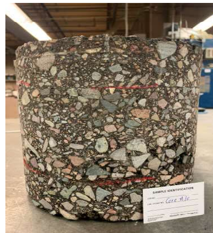
B10 Core Thickness: 8.8-in Top: 2.2-in, Middle 4.2-in, Bottom: 2.4-in.
