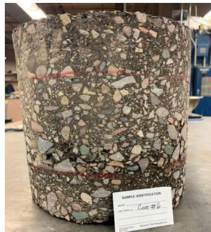
B6 Core Thickness: 9.0-in Top: 2.2-in, Middle 4.2-in, Bottom: 2.6-in.
