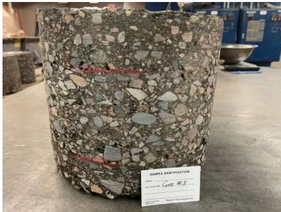
B3 Core Thickness: 8.5-in Top: 2.2-in, Middle 4.1-in, Bottom: 2.2-in.
