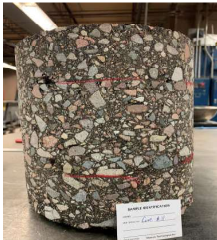
B11 Core Thickness: 9.4-in Top: 2.3-in, Middle 4.1-in, Bottom: 3.0-in.
