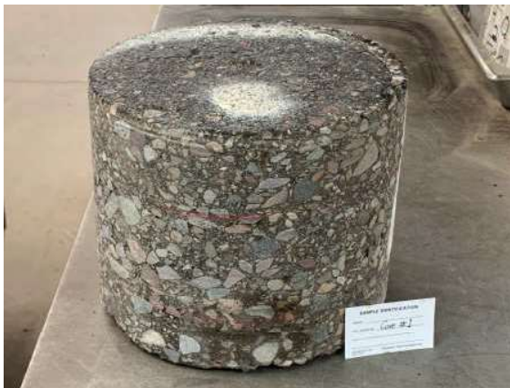
B1 Core Thickness: 8.1-in Top: 2.4-in, Middle 3.3-in, Bottom: 2.4-in.
