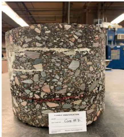
B7 Core Thickness: 9.1-in Top: 1.9-in, Middle 4.3-in, Bottom: 2.9-in.
