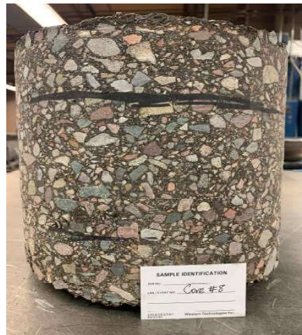
B8 Core Thickness: 9.0-in Top: 2.3-in, Middle 3.9-in, Bottom: 2.7-in.
