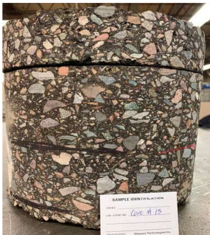
B15 Core Thickness: 8.9-in Top: 2.1-in, Middle 3.4-in, Bottom: 3.4-in.
