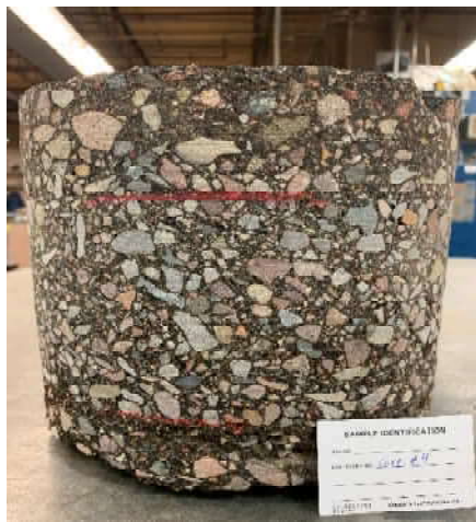
B9 Core Thickness: 7.7-in Top: 1.6-in, Middle 4.1-in, Bottom: 1.9-in.
